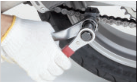
15a. Hold the hexagon part of the tool body by with a 27mm closed in wrench, and the bolt head with a 19mm closed end wrench; turn clockwise until the flare part of the pin head makes contact with the surface of the side plate.
