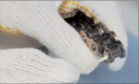
8a. Before installing the connecting link, be sure to put a heavy coat of the supplied grease into the holes of the bushings of the new chains' links, and on the surface of the connecting link's pins. If you are installing an O-Ring or X-Ring® chain, don't forget to put heavily greased O-Rings or X-Rings on the pins between the sideplates on both sides of the chain.
