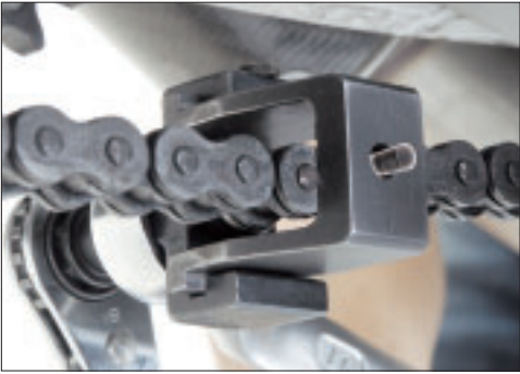
5a. Turn 19mm wrench clockwise on the tool's Hexagon bolt head to push the pin completely out.
