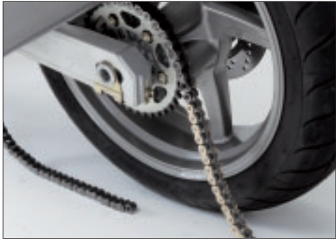
6a. After pushing the pin out, disassemble the chain tool from the chain.
