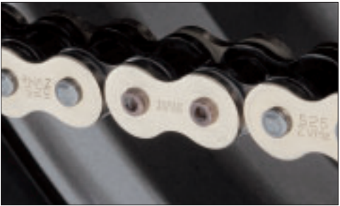
12a. After pressing the sideplate on, disassemble the chain tool and remove it from the chain. The next step is to flare out the pins heads for ZJ (Rivet type) or installing the slide clip for the FJ (Cliptype) master link.
