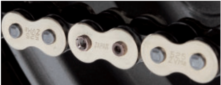
All ZJ rivet style cover plates are press-fit.
