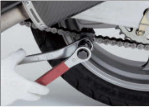
4a. Use a 27mm closed in wrench to hold firm the body of your chain tool while using a closed end 19mm wrench on the tool's hexagon bolt head to tighten. It will be easier to tighten the bolt if you position your wrenches 30° apart.
