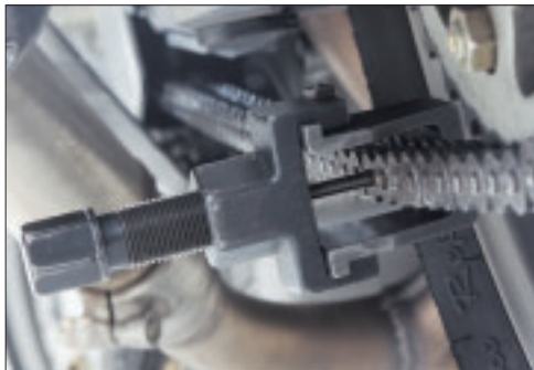
3a. To align the tool's Cutting pin with the chosen pin head, turn the tool's large bolt head clockwise "by hand" until the Cutting pin comes in contact with the pin head. At this point, make sure that the cutting pin is lined up with the center of the pin you wish to push out.
