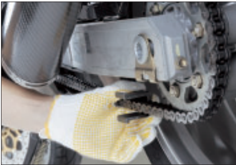
1a. Before cutting your chain, loosen it using your motorcycle's rear wheel adjusters. Position your KM500R over your chain on the bottom side of your swingarm; cut the pin on the right side of the link you choose first. If your chain has a master link, it is easier to cut the chain at the master link.
