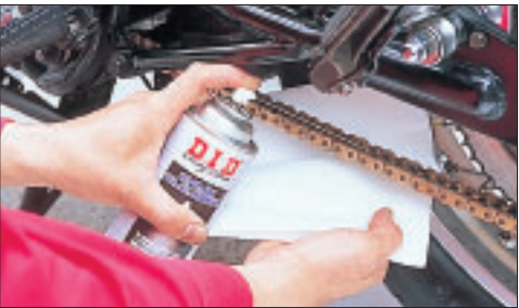
7a. Before spraying on the chain lube, put a tray under the chain and hold a towel behind the chain to prevent overspraying on the motorcycle. Put the motorcycle on stand to allow rotating the rear wheel. When spraying on chain lube, keep the can nozzle a distance of between 2" to 4" away from the chain. While spraying, rotate the rear wheel by hand to coat the entire chain.
