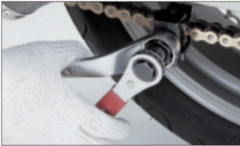
11a. Hold the hexagon part of the tool body with a 27mm closed end wrench and turn the bolt with a 19mm closed in wrench clockwise until the top of the pins make contact with the groove in the Plate holder.
