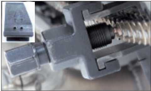
14a. Set aside the Plate Holder and set the pin on the tool body to the B position to flare out the pin heads.
